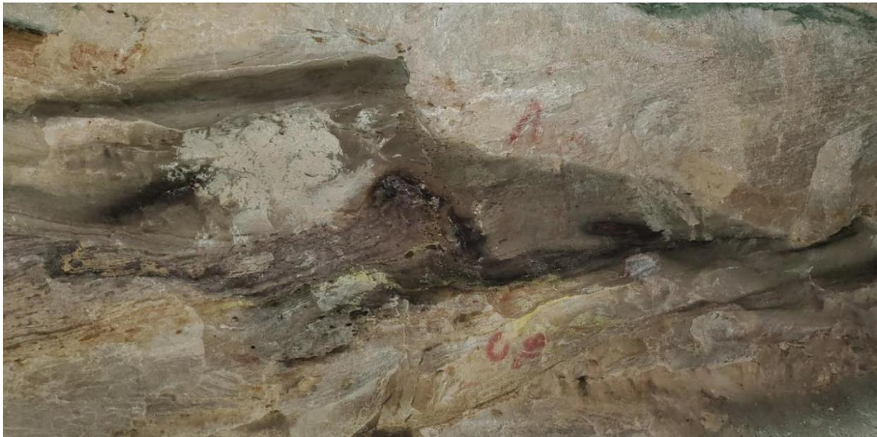
Figures 3 and 4 – The Yellow Circle underground workings have many instances where vanadium mineralization is visible, denoted by the dark grey to black coloration.
