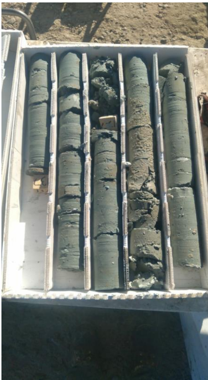
Figure 1 and 2 – photos of drill core derived from Hole #1. Currently at approximately 227ft (69m) in depth and continuing to drill.
